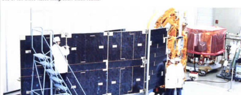
One of ten Class 10,000 integration clean rooms.
