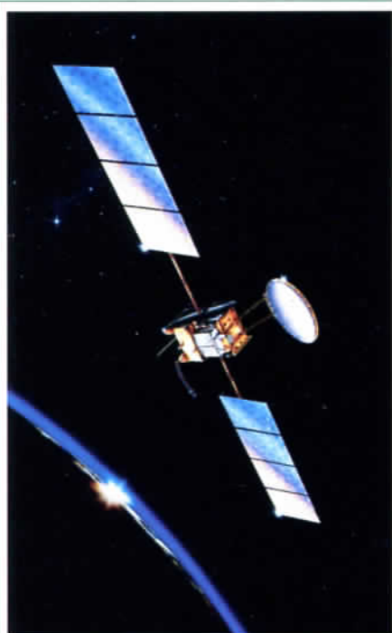
This direct broadcast satellite carries three 200-watt transponders.
