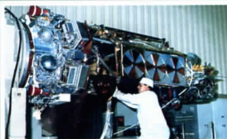
Final inspection of a DMSP Block 5D2.
