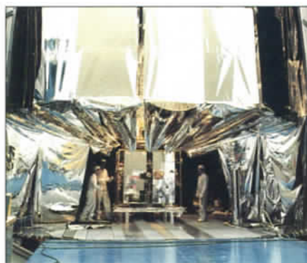
Aurora II is prepared for thermal-vacuum test.
