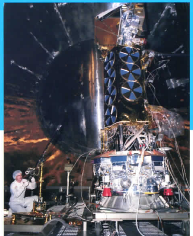
Preparation of an Advanced TIROS-N for thermal vacuum testing.
